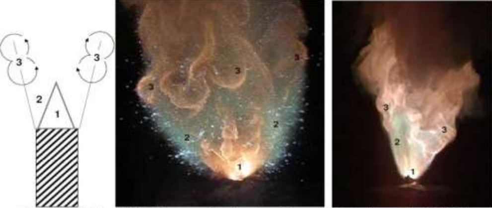
Fig. 8. Model for MTV flare combustion (a) with real photo-image for MTV flame (b)
