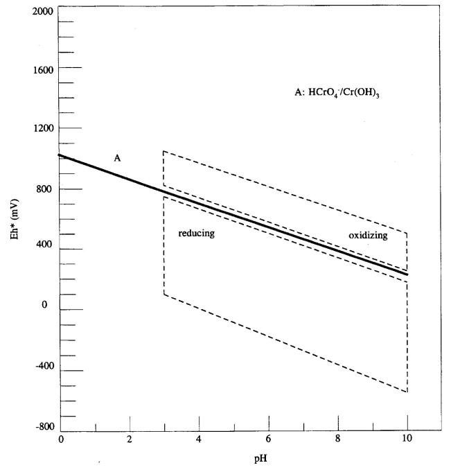
\* Note the Eh values plotted on this diagram are corrected for the reference electrode voltage: 244 mV units must be added to the measured value when a separate calomel electrode is used, or 199 mV units must be added if a combination platinum electrode is
