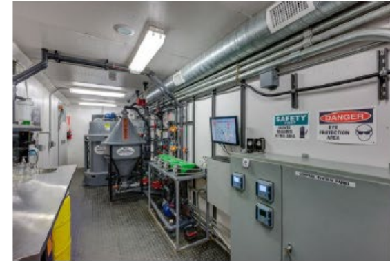
PFAS in Raw Sewerage: Electro-coagulation + SAFF
