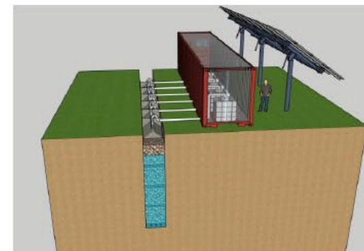
Trench Based Downhole Foam Fractionation, USA
