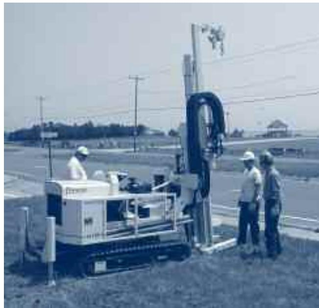
*Geoprobe for soil and groundwater sampling*
