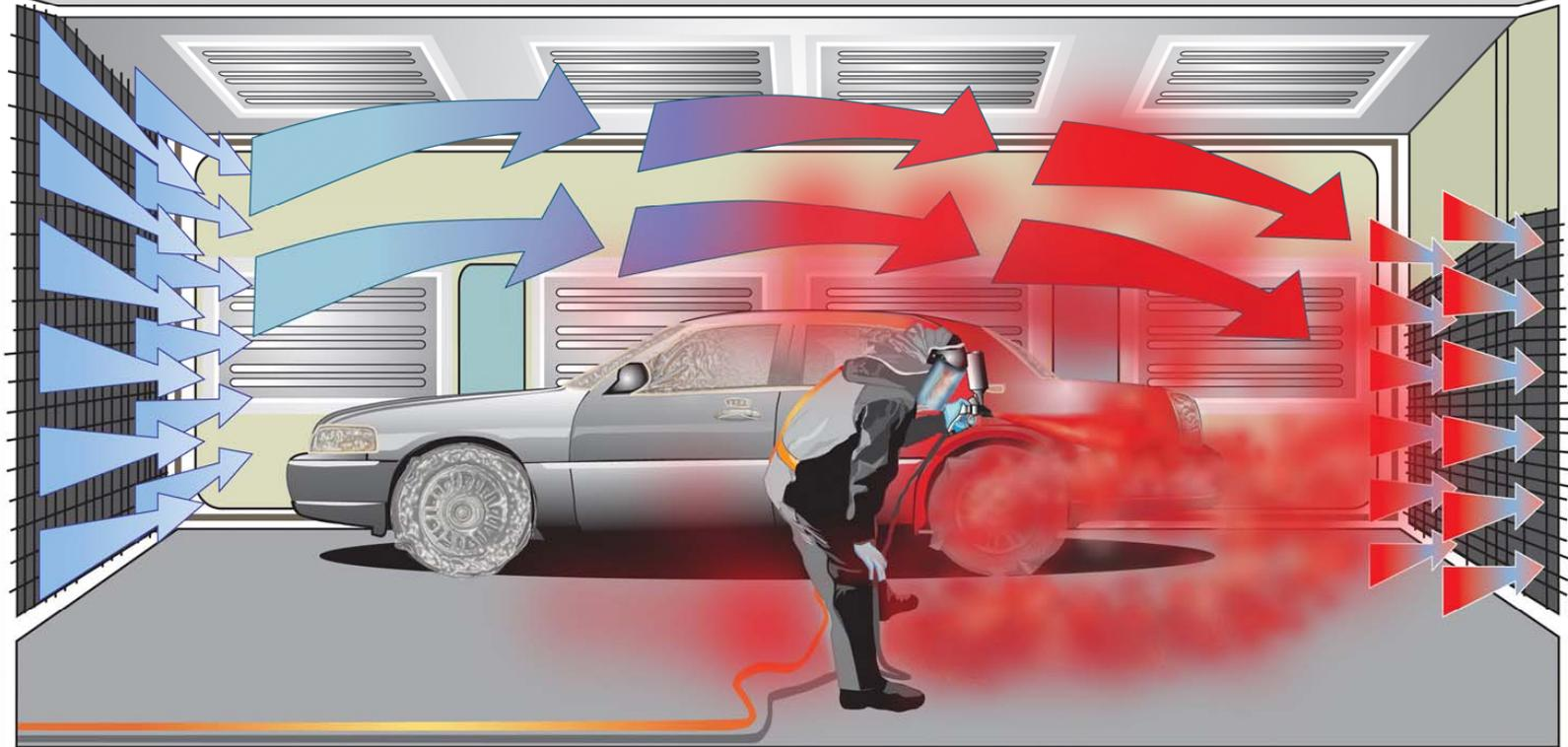
**Filtered air enters at left side of booth and exits through right side.**
