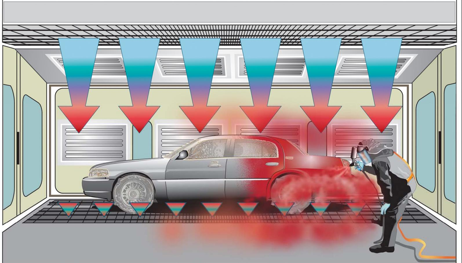
Filtered air enters at ceiling of booth and exits through the floor.
