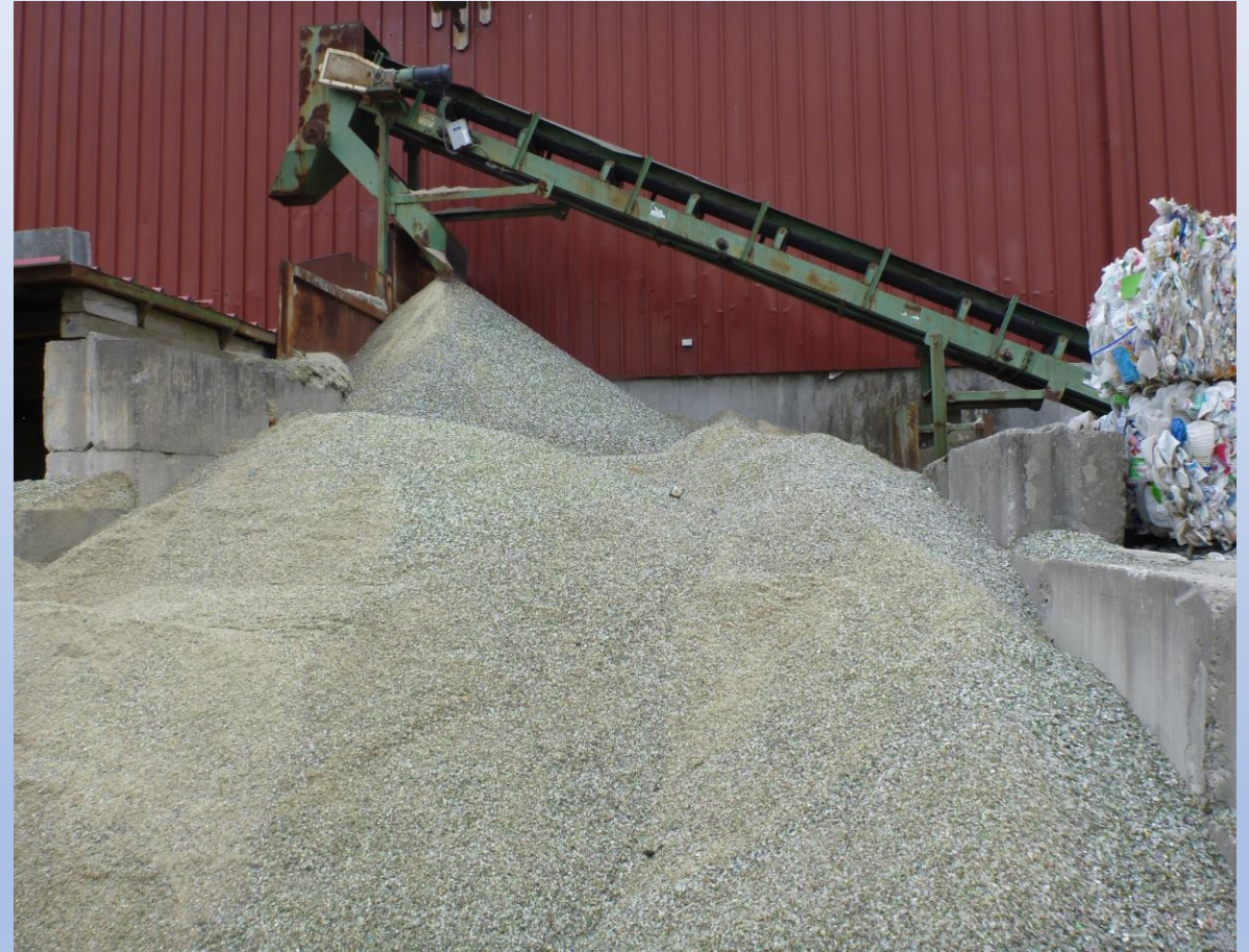
PGA produced by Windham County Solid Waste District MRF
