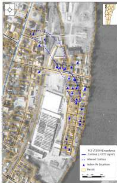
Figure 2: Site Map With Indoor Air Quality Results for tetrachloroethene (aggr) Windsor, Vermont
