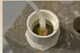
Cox-Colvin Vapor Pin with Water Dam
