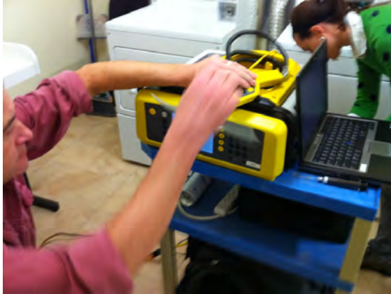
Instant results using portable analyzer (HAPSITE)
