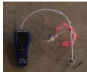
4. Sub-slab gas and differential pressure monitoring
