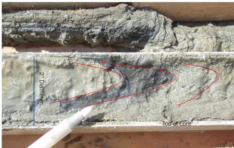
Extreme Deformation in Silt Unit.
