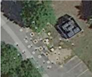
Dense Push Array at Highly Characterized DNAPL Source Zone
