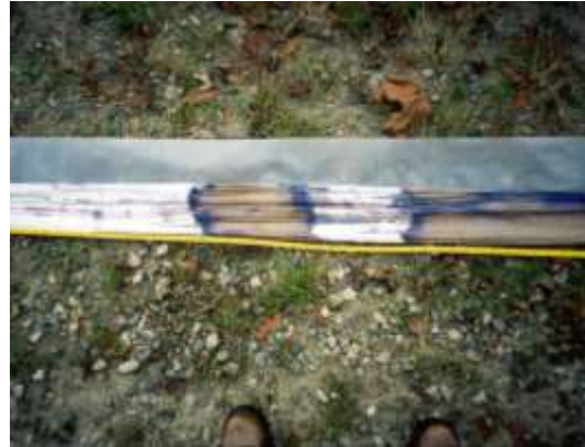
Stains Caused by Reactive Dye Indicate Presence of DNAPL
