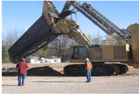
One-Pass Trencher used to install the 850-ft long PRB at West Valley, New York Courtesy, De Wind One Pass Trenching and ITRC
