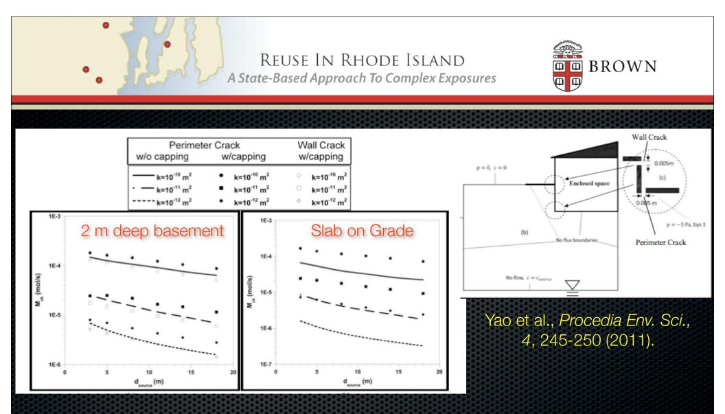
Slab-on-grade COC entry rate ( $M_{ck}$ ) is much more sensitive to capping around building than is basement foundation (10m x 10 m foundation, 5 m apron)
