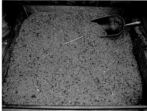
Picture 4 – 1/8-Inch Crushed Glass Sample Prior to Separation.
