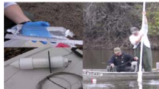
Peepers consisted of dialysis tubing filled with reagent grade water placed into a protective sheath, and then inserted to a depth of 10 cm into the sediment
