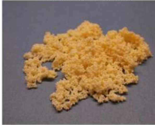
Sorbix A3F A strong base anion exchange resin
