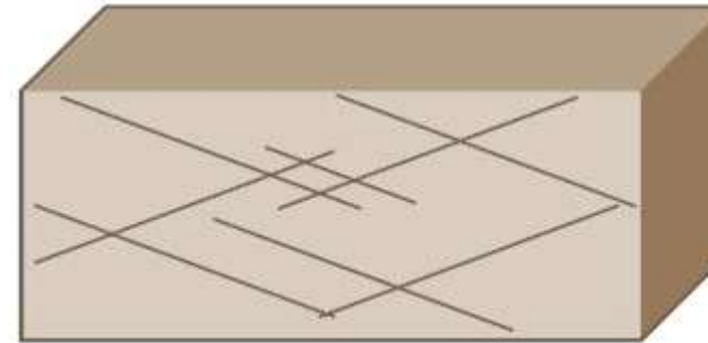
(V) Fracture Media with High Matrix Porosity (e.g. limestone, sandstone or fractured clays)
