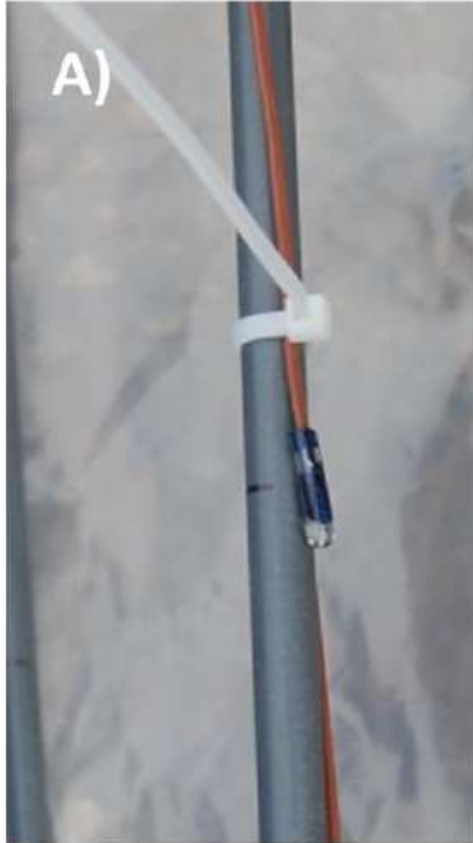
Thermocouple on temperature monitoring “stick”
