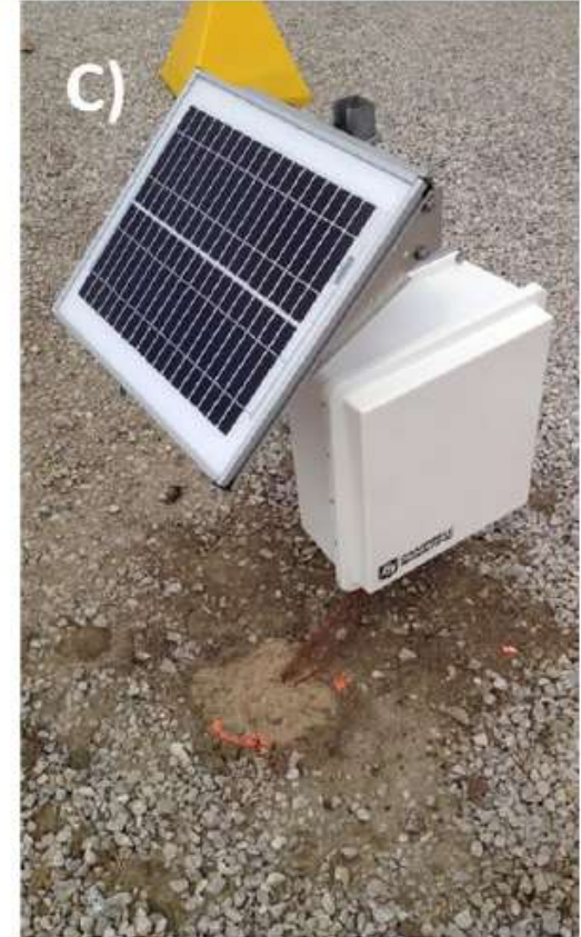
Solar power supply and weatherproof box with data logger and wireless communications system.
