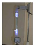
Mercury Spectral Tube in Action
