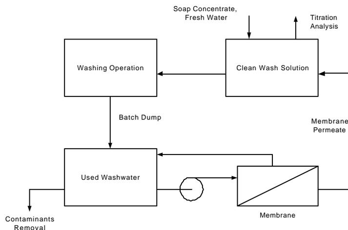
**Figure 2: Aqueous Cleaner Recycling – Example Batch System Configuration<sup>13</sup>**
