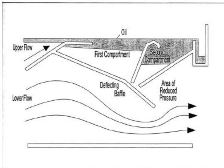
**Figure 1: Suparator™ Oil Separation Compartment**<sup>8</sup>
