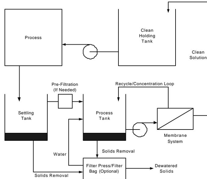
**Figure 3: Aqueous Cleaner Recycling – Example Continuous System Configuration<sup>14</sup>**
