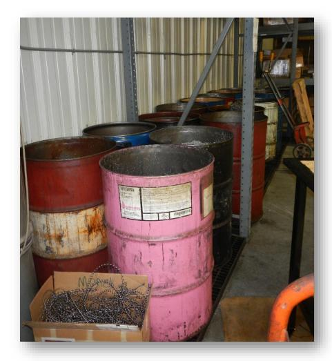
Coolant and tramp oil are drained from waste metal and collected before the metal is shipped for recycling. Smaller shops gravity drain the chips.
