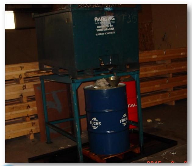
Another chip draining set up. These chips were too large to spin in a centrifuge.
