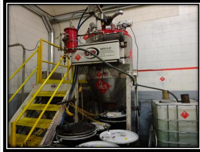
Waste Pumped to Distillation Unit for Recycling
