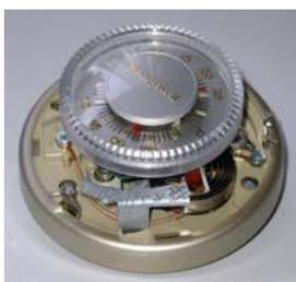
Mercury Switch inside Thermostat
