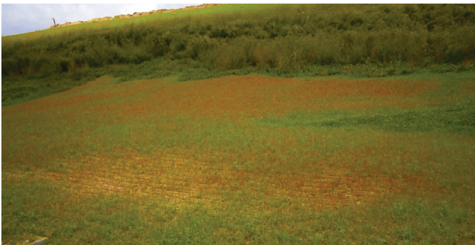
Distressed Vegetation Due to Landfill Gas
