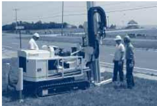
*Geoprobe for soil and groundwater sampling*
