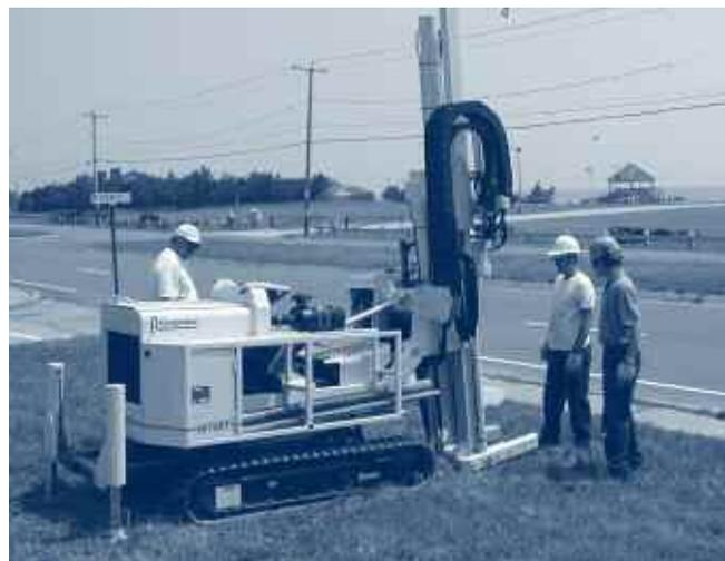
*Geoprobe for soil and groundwater sampling*
