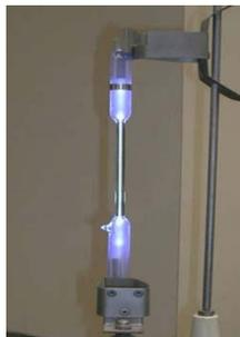
**Mercury Spectral Tube in Action**
