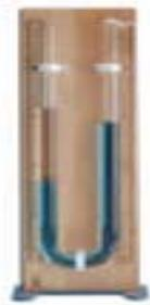
**U-tube Manometer filled with Blue Liquid**
