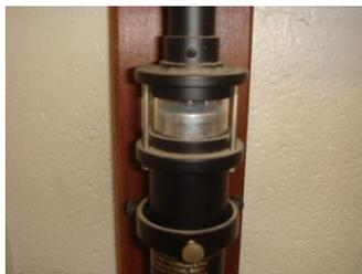
Close-up of a Mercury-Filled Barometer
