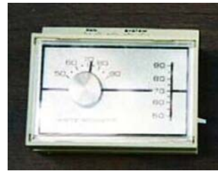
Mercury Thermostat Source: NEWMOA
