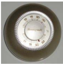
Mercury Thermostat Source: NEWMOA
