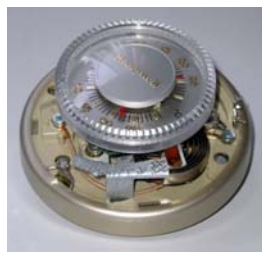
Mercury Switch inside Thermostat Source: Wikipedia
