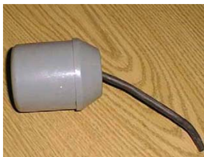
Mercury Float Switch used in a Sump Pump Photo Source: Vermont Agency of Natural Resources
