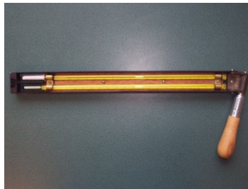
Mercury Sling Psychrometer; Source: Wikipedia
