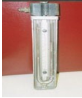
Mercury Dairy Manometer; Source: Cuoco & Cormier Engineering
