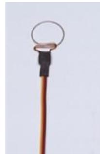
Mercury Strain Gauge for Digits (fingers and toes)
