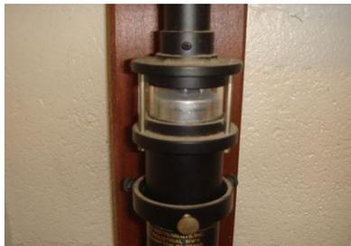
Close-up of a Mercury-Filled Barometer; Source: NEWMOA
