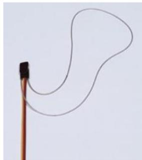
Mercury Strain Gauges for Leg
