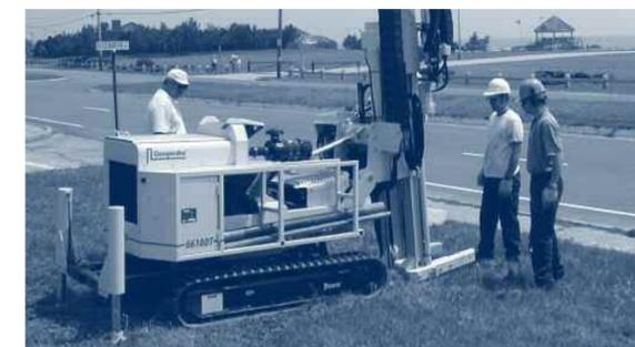
Geoprobe for soil and groundwater sampling
