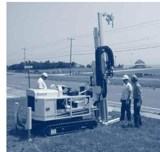
Geoprobe for soil and groundwater sampling
