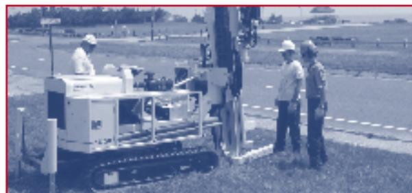
Geoprobe for soil and groundwater sampling
